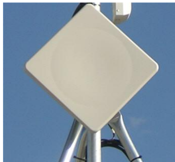
Figure 18 -- Panel antennas are most often used for point-to-point applications
